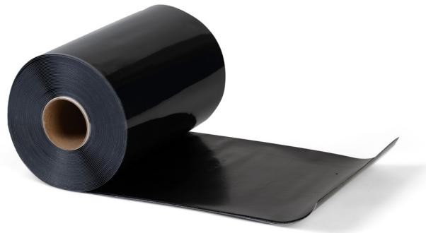
Effisus Bond FT Tape consists of an uncured EPDM membrane that has been laminated to a pressure-sensitive tape adhesive of 0,64 mm thickness, integrating a proven peel & stick technology. The Effisus Bond FT tape is extremely flexible, malleable and can be formed to fit irregular shapes and surfaces. Once cured, the tape is highly resistant to moisture, UV, temperature variations, and structural movements.
