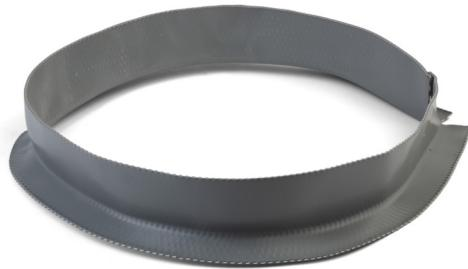
Effisus Multishapper is a stretchable, flexible and conformable L shaped curb, based on polymer rubber with an interior aluminium reinforcement, that can be easily shaped without requirements for special tools, to obtain a curb with any geometry desired. Final curb is closed easily in one step (no tools) with a metal locking clip and is intended to be filled with liquid or semi-liquid materials. Resistant to ice, stagnant water and ozone stable.
