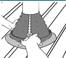
To assist in locating the clip into the pocket, place a hand behind the Effisus Stopper MR seam.
