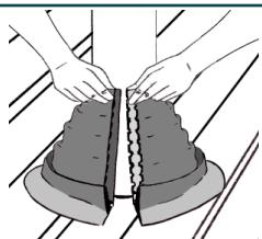
With the clip in the downstream position, wrap the top of the cone around the pipe.
