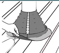
Using your hands, apply pressure to the base of the Effisus Stopper MR so that it conforms to the contours of the roof panel, adjusting it to the roof corrugation.
