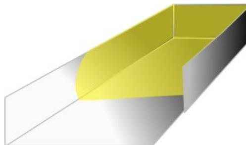
3. Cut the Effisus Alltitegutter Membrane into the required dimensions. Cut the protective foil according with the gutter dimensions and areas as seen on the side picture (bottom, sides, etc.) – make sure to cut the membrane below the protective foil.
