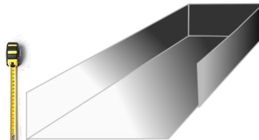
2. Apply the Effisus Primer 9800 into the entire gutter surface with a roll or brush. Allow the primer to dry off before adhering the Effisus Alltitegutter Membrane.
