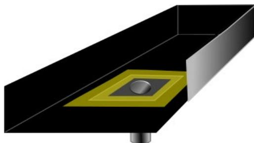
2. Position Effisus Bond FT Tape over primed area around the drain outlet perimeter. Apply Bond FT tape with two bands as shown in the two images on the right, as indicated in (1) and (2), with an overlap of a minimum of 75mm. Press down and form Effisus Bond FT Tape by hand. Roll the flashing with a 50mm wide silicone roller. The overlap of the tape on the Effisus Alltitegutter Membrane should be done with a minimum of 75mm.
