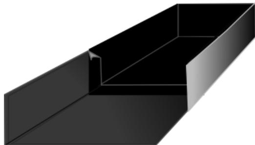
2. Apply a layer of Effisus Primer RED+ with a minimum width of 150mm, centered with the joint. Allow the primer to dry off before adhering the overlapping joint tape.
