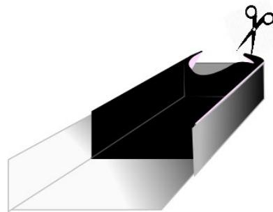
2. Remove the protective foil and adhere the membrane to the gutter on the intended position. Press it with a silicone roll in order to promote the adherence of the membrane.
