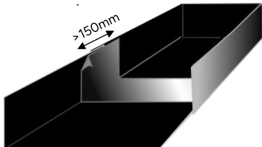
4. Seal the entire perimeter of the Effisus Bond FT Tape with a Effisus Bonding KF+P bead with approx. 5mm diameter.
