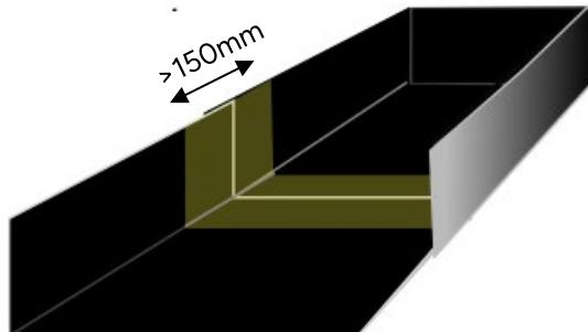
3. Adhere the Effisus Bond FT, centered with the joint, removing the protective foil progressively and pressuring the tape with a silicone roll. Apply the Effisus Bond FT Tape with no less than 150mm, with a minimum of 75mm for each side of the membrane overlap joint.
