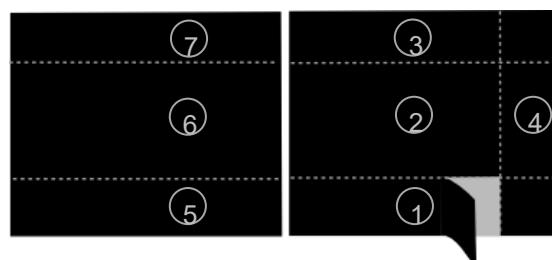
4. Adhere the Effisus Alltitegutter membrane to the gutter, on the intended final position. Roll it with a silicone roll in order to improve adhesion and make sure that the entire membrane surface is adhering to the gutter surface.
