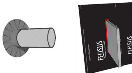
Figure 7 – Sealing service penetrations and cladding fixing perforations.
