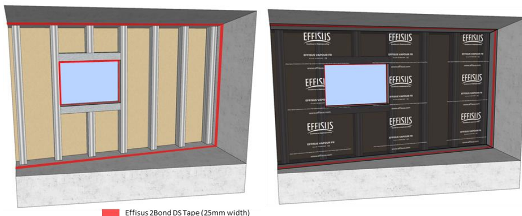
Figure 6 - Effisus Vapour FR Membrane – Overlapping Joints.
