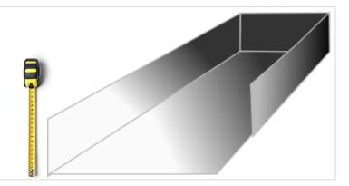
Apply the Effisus Primer 9800 into the entire gutter surface with a roll or brush. Allow the primer to dry off before adhering the Effisus Alltitegutter Membrane.
