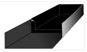
2. Apply a layer of Effisus Primer RED+ with a minimum width of 150mm, centered with the joint. Allow the primer to dry off before adhering the overlapping joint tape.
