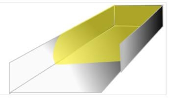
3. Cut the Effisus Alltitegutter Membrane into the required dimensions. Cut the protective foil according with the gutter dimensions and areas as seen on the side picture (bottom, sides, etc.) – make sure to the cut the membrane below the protective foil.
