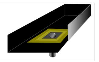
2. Position Effisus Bond FT Tape over primed area around the drain outlet perimeter. Apply Bond FT tape with two bands as shown in the two images on the right, as indicated in (1) and (2), with an overlap of a minimum of 75mm. Press down and form Effisus Bond FT Tape by hand. Roll the flashing with a 50mm wide silicone roller. The overlap of the tape on the Effisus Alltitegutter Membrane should be done with a minimum of 75mm.
