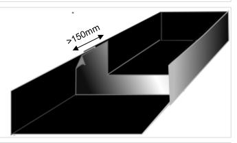
4. Seal the entire perimeter of the Effisus Bond FT Tape with a Effisus Bonding KF+P bead with approx. 5mm diameter.
