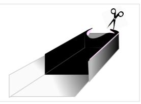
2. Remove the protective foil and adhere the membrane to the gutter on the intended position. Press it with a silicone roll in order to promote the adherence of the membrane.
