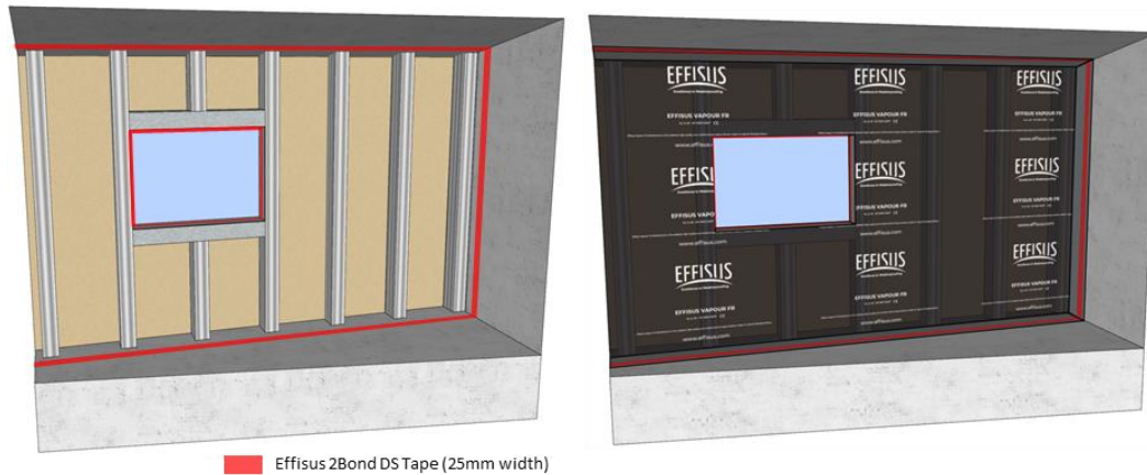
Figure 5 - Effisus Vapour FR Membrane – Perimeter sealing.
