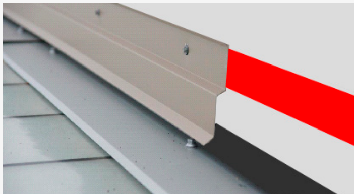
5- Sealing perforations when fixing border guards
