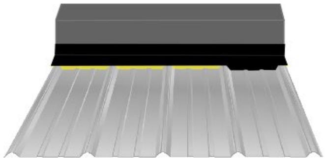
4. Press the entire bonding area with a silicone roll in order to promote a perfect adherence between the tape and the substrate. Finish the application by applying a bead of Effisus Bonding KF+P to the entire perimeter of the Effisus Bond FT Tape.
