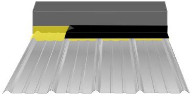
3. With hand, or with help of a silicone roll, start moulding/adjusting the tape to the corrugated surface. Make sure to not stretch the tape too much on a single point (ex: corners), in order to avoid any risk of damaging it.
