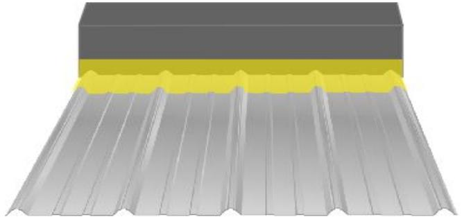
2. Start bonding the tape to the substrate by progressively taking off the protective foil and bonding the tape flat without forcing it to follow the corrugated surface.
