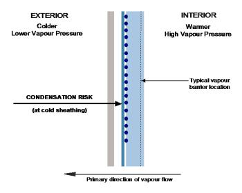
Figure 2 – Vapour flow in cold climates
