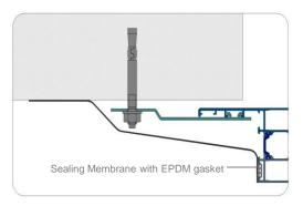
Fig. 2 Sealing membrane with clip-in gasket
