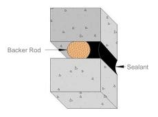
Fig. 1 Standard sealing detail with sealant and backer rod
