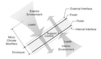
Fig. 1 Building enclosure and its functions (1)
