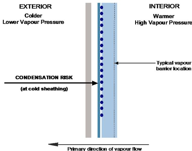
Figure 2 – Vapour flow in cold climates
