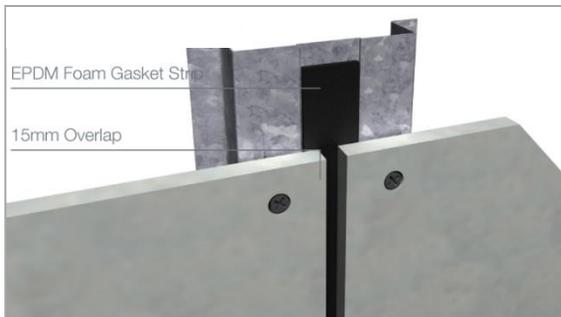
Fig. 3 Sealing detail with foam gasket strip
