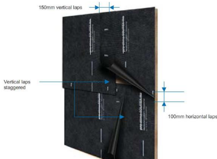
Fig. 4 Æ Effisus Breather Membrane Æ Overlapping Joints
