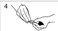
Effisus 2Bond GO Tape also can be used as a putty. Remove both release liners and roll into a rope. Place Effisus 2Bond GO over the gap and mold to the seal the opening.
