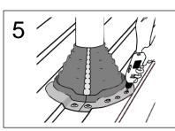
Press the Effisus Stopper into the roof, adjusting this to the roof corrugation with your hands.
