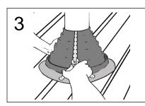
To assist locating clip into pocket, place an hand behind the Effisus Stopper MR seam.
