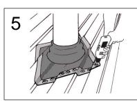
Slide down the Effissu Stopper MR into the intended position. Start fastening the Effisus Stopper MR to the roof with one screw at 2 opposite sides of the Effisus Stopper base.
