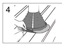
Using your hands apply pressure to the base of the Effisus Stopper MR into contours of the roof panel, adjusting this to the roof corrugation.
