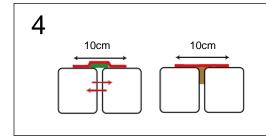
If movement is expected, apply the Effisus 2Bond DS Tape in the joint first and then apply the Effisus Easyrepair Membrane. This combination is better for absorbing movements than one layer of Effisus Easyrepair Membrane.
