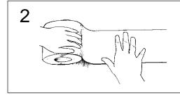
There mustn't be less than 2.5cm of Effisus Easyrepair Membrane on each side of the joint.
