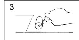
Seams between Effisus Easyrepair Membranes should have a minimum overlap of 100mm.
