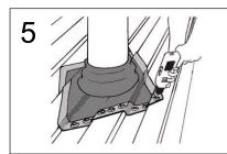
Slide down the Effissu Stopper MR into the intended position. Start fastening the Effisus Stopper MR to the roof with one screw at 2 opposite sides of the Effisus Stopper base.
