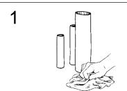
Remove all previously applied caulk, mastic, cement, asphalt and other contaminants from penetrations with a wire brush to ensure proper bonding.
