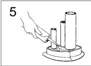
Pour the Effisus Stopper 1-P Sealant: fill the Effisus Stopper EC/CE Curb with Effisus Stopper 1-P Sealant up to the curb top. Tool off to a smooth surface.
