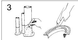
Seal the base of each penetration with the Effisus Stopper M-1 Sealant and coat the penetrations surfaces up to three inches above the roofline.
