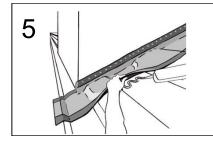
Fold the Effisus Cobra Membrane back and apply a continuous bead of Effisus Block JP Sealant on the roof (this bead should be applied on the position where the bottom edge of the Membrane will be fastened to the roof).
