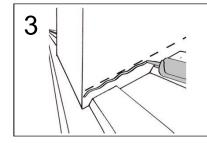
Apply a continuous bead of Effiisus Block JP Sealant below the guideline marked previously on point 2.
