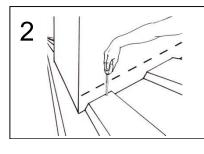
Start the installation of the Effisus Cobra Membrane from the bottom of the duct (lower side of the roof slope).
