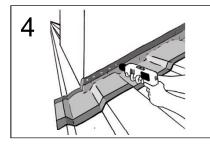
Secure the Effisus Cobra Membrane to the duct following the guideline previously marked on point 2.
