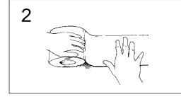
To apply the Effisus 2Bond DS Tape, remove one side of the release liner and apply to the surface to be protected or bonded. Rub or roll with pressure using your hand or a steel roller to activate bonding process. Remove the second release liner and apply second surface to tape, apply pressure.
