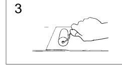
Seams between Effisus 2Bond DS Tapes should have a minimum overlap of 100mm. Adhere the top Effisus 2Bond DS Tape over the bottom Effisus 2Bond
