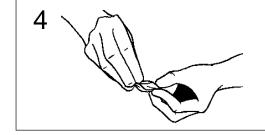
Effisus 2Bond DS Tape also can be used as a putty. Remove both release liners and roll into a rope. Place Effisus 2Bond DS over the gap and mold to the seal the opening.
