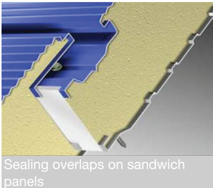
Sealing overlaps on metal plates
