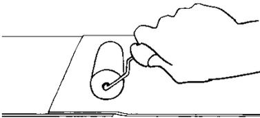
Seams between Effisus Easyrepair Membranes should have a minimum overlap of 100mm. Adhere the top Effisus Easyrepair Membrane over the bottom Effisus Easyrepair Membrane. Roll with pressure using a steel roller, to activate bonding process.
