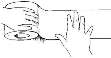
There mustn't be less than 2.5cm of Effisus Easyrepair Membrane on each side of the joint. Install Effisus Easyrepair Membrane over the repair area, removing the release liner gradually, to prevent contamination of the adhesive prior to application. Roll with pressure using a steel roller, to activate bonding process. Apply gently and without tension.
